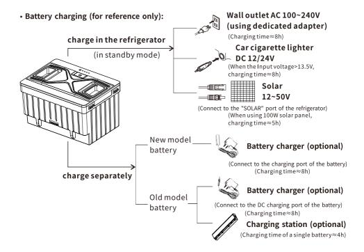
**Note:** It is suggested to switch off the refrigerator when charging the battery (the power supply may mainly power the compressor when the refrigerator is running).
